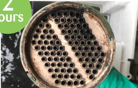
Volvo Heat Exchanger after 2 hour treatment of CleanScale.
