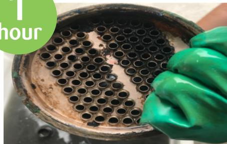
Volvo Heat Exchanger after 1 hour treatment of CleanScale.
